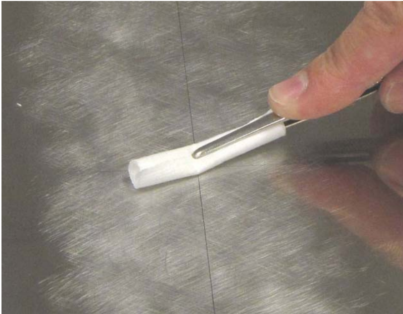
Fig. 3.2: Final cleaning of the installation point
