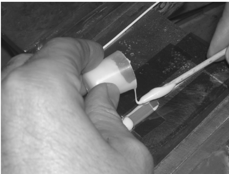
Fig. 7.18: Applying the X60 adhesive
