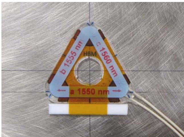
Fig. 5.1: Aligning the optical rosette on the double marking cross
