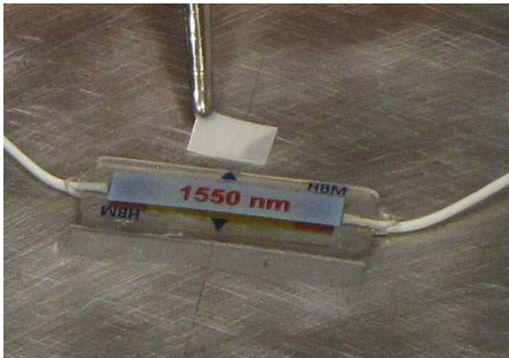
Fig. 4.2: Applying the adhesive tape to the measurement point
