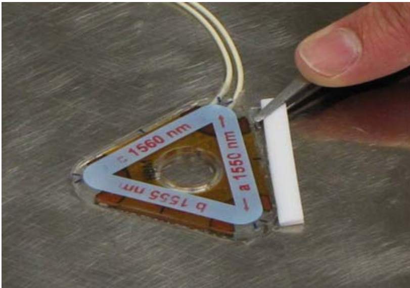
Fig. 5.10: Removing the Teflon installation aid
