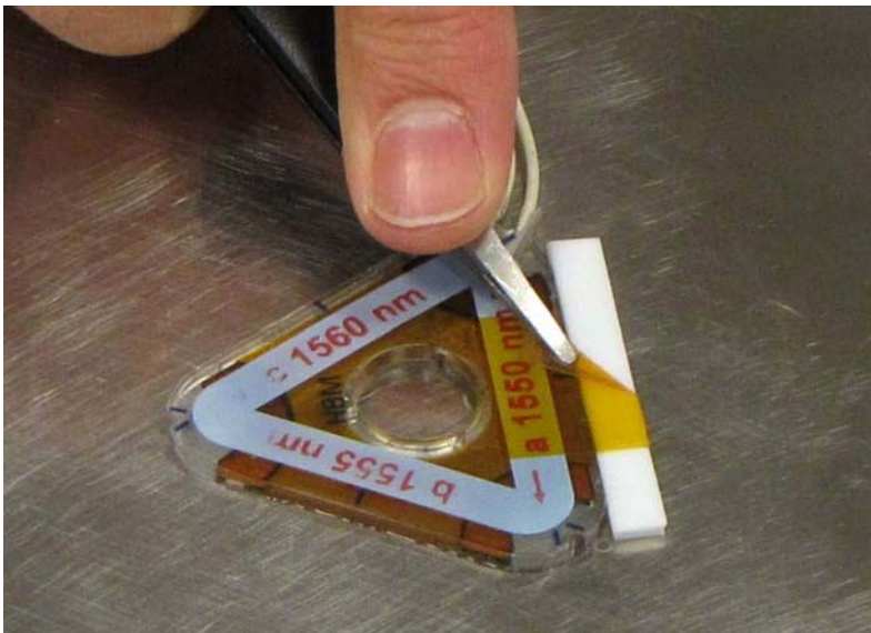
Fig. 5.9: Removing the second adhesive tape
