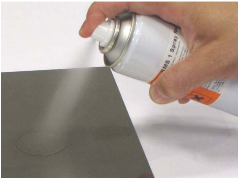
Fig. 2.1: Spraying the measuring point with 1-RMS-SPRAY
