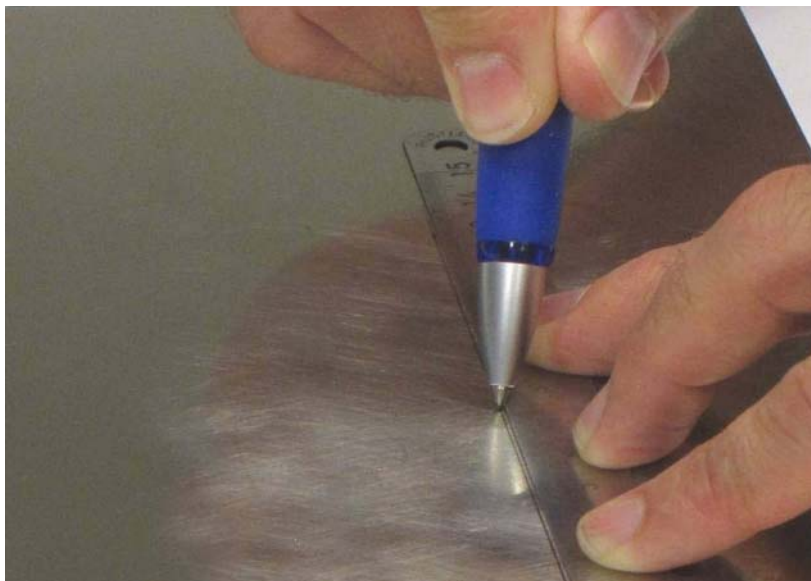
Fig. 3.1 Marking the marking lines
