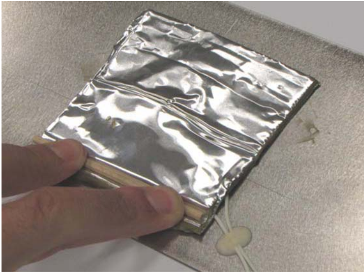
Fig. 6.2: Applying and pressing down the covering foil ABM75
