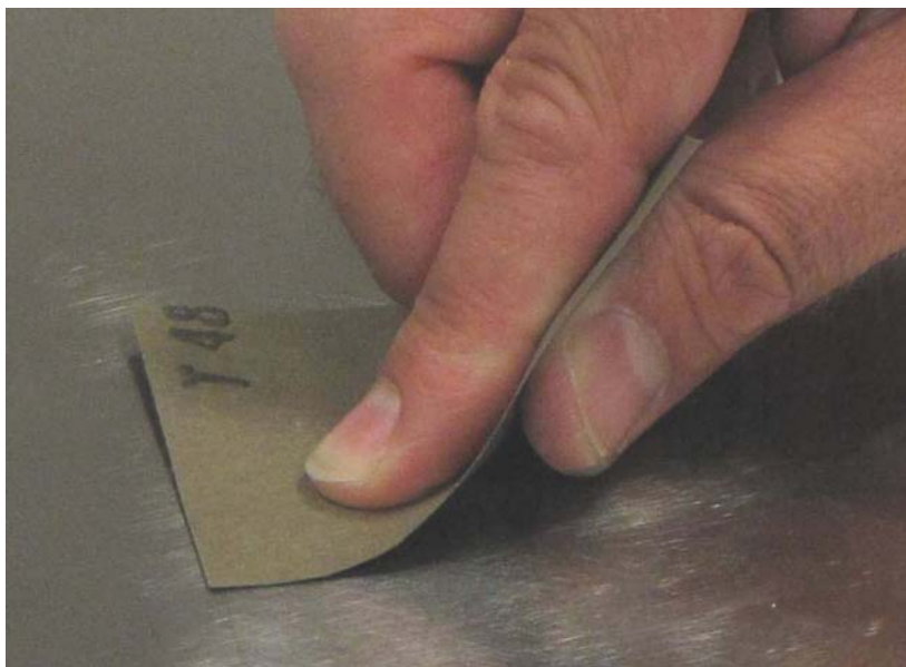
Fig. 2.3: Roughening the surface of the measuring body
